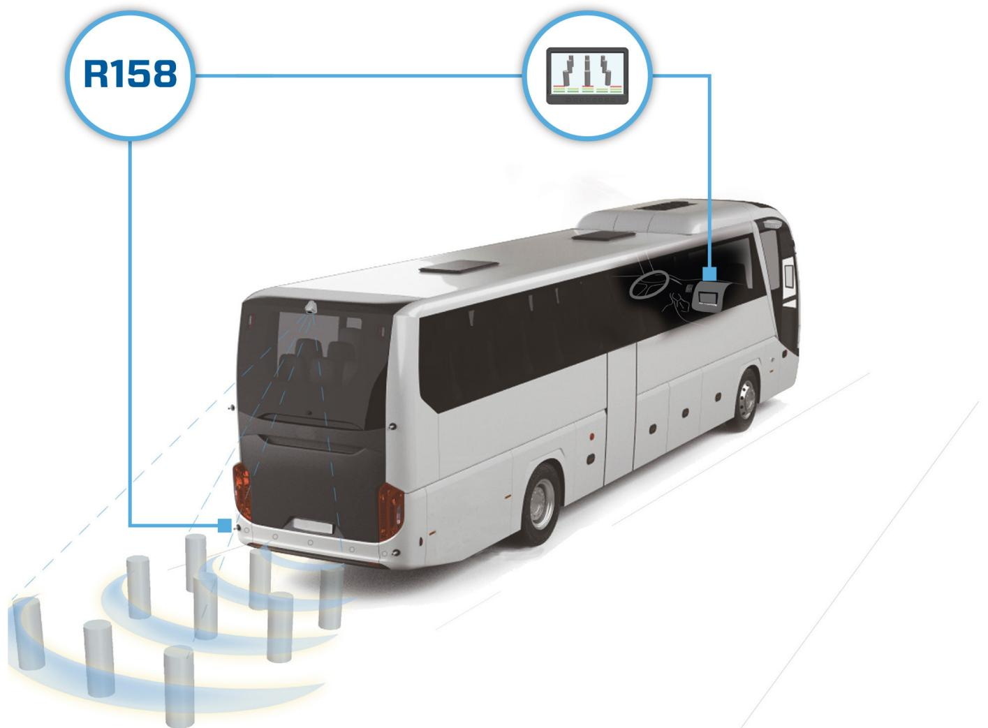
The monitor, in reverse gear, warns of object detections
